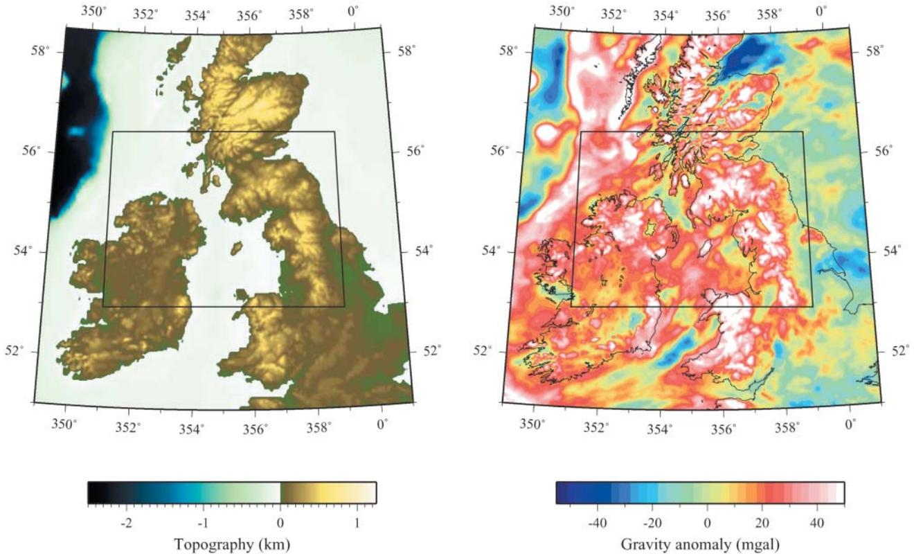
**Fig. 1.** (a) Topography of British Isles taken from ETOPO5/GETOPO30 dataset (ETOPOS Database 1988; Smith & Sandwell 1997). (b) Combined onshore/offshore free-air gravity map (BGS 1997). In both cases, data were interpolated onto a grid in an oblique Mercator Projection with axis at  $-90^\circ$  longitude and mesh size of 30 km. Admittance calculations were carried out for this map region but we also analysed data from the smaller outlined box.
