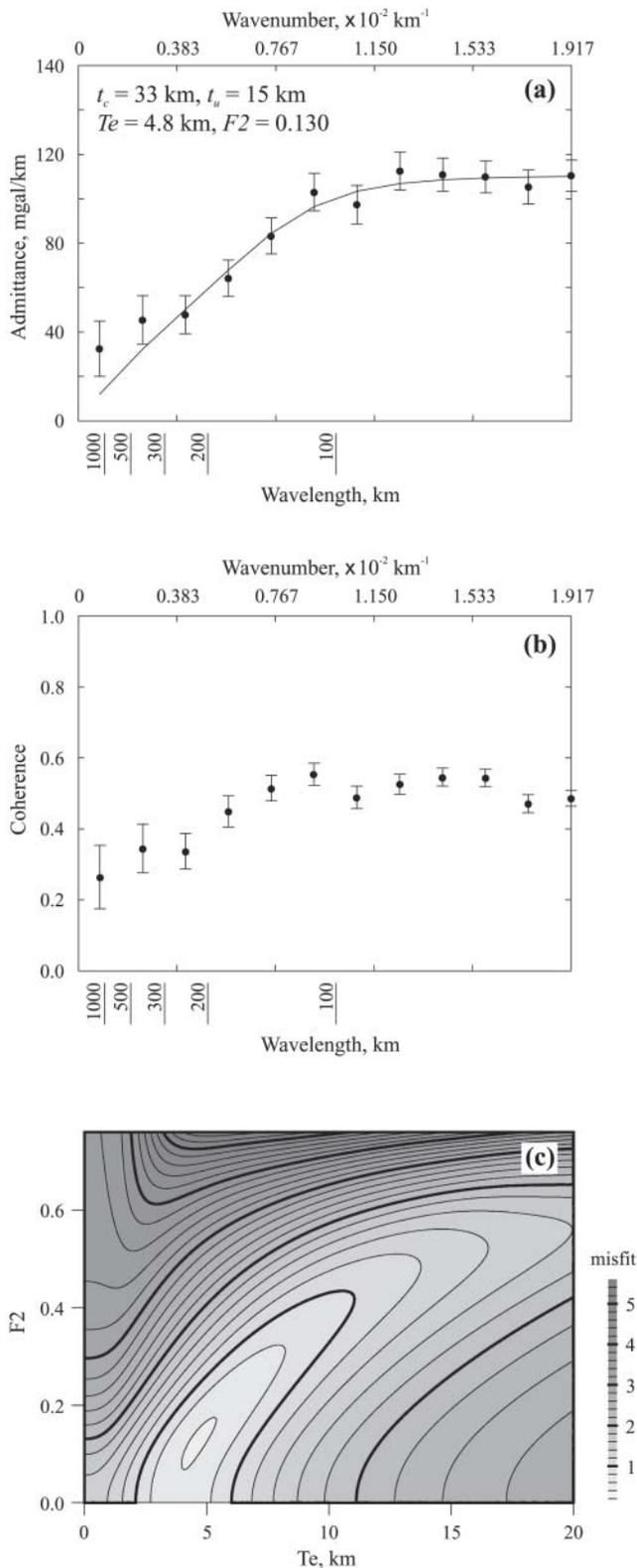
**Fig. 2.** Admittance and coherence calculations for map region of Figure 1. (a) Vertical error bars are observed values of  $Z_f(k)$  calculated from topography and free-air gravity; the solid curve is the best-fitting theoretical  $Z_f(k)$  determined by varying  $T_e$  and  $F_2$ . (b) Observed coherence between free-air gravity anomaly and topography. (c) Contour plot of misfit function,  $H(T_e, F_2)$ . Note positive trade-off between  $T_e$  and  $F_2$ .
