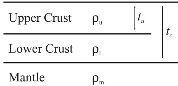
**Fig. 3.** Sketch of model used to calculate response to surface and internal loads.  $t_c = 33$  km;  $t_u = 15$  km;  $\rho_u = 2.67$  Mg m $^{-3}$ ;  $\rho_l = 2.9$  Mg m $^{-3}$ ;  $\rho_m = 3.33$  Mg m $^{-3}$ . Figure constructed using Generic Mapping Tools of Wessel & Smith (1998).
